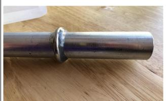
**Step -2**: Mix a small amount of the two-part epoxy, and secure the ring as shown. Or This can be welded.
